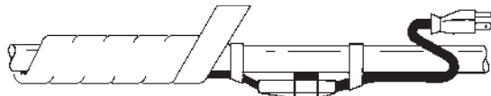
Automatic Pipe Heating Cable on Metal Water Pipe (See “Special Notes for Plastic Pipes” below.)
