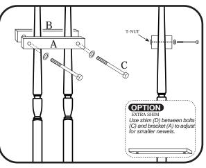
Insert bolt with washer through clamp and screw into T-nut on opposite clamp. The clamp with the T-nut should be on the outside of the post. Mount gate according to instructions. Use shim if necessary to ensure level gate installation.
