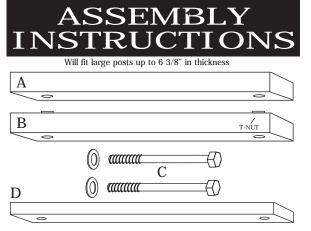
This wood clamp provides a means for attaching your gate to a large post or spindles without damaging the post with screws. Please follow these procedures to install a CARDINAL GATE.
