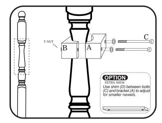
Insert bolt with washer through clamp and screw into T-nut on opposite clamp. The clamp with the T-nut should be on the outside of the post. Mount gate according to instructions. Use shim if necessary to ensure level gate installation.
