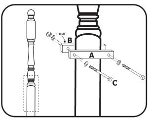
Insert bolt with washer through clamp and screw into T-nut on opposite clamp. The clamp with the T-nut should be on the outside of the post. If threaded bolt extends through **B** block, add lock nut (and extra washers if needed) for safety. Mount gate according to instructions.
