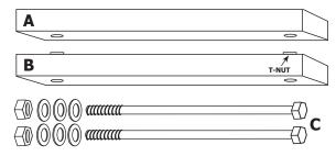
Wood Clamps provide a means for attaching your gate to a post without damaging the post with screws. Please follow these procedures to install a CARDINAL GATE.
