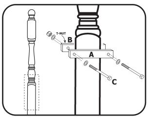
Insert bolt with washer through clamp and screw into T-nut on opposite clamp. The clamp with the T-nut should be on the outside of the post. If threaded bolt extends through **B** block, add lock nut (and extra washers if needed) for safety. Mount gate according to instructions.
