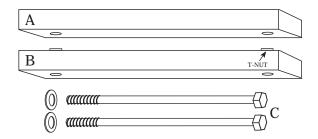
Wood Clamps provide a means for attaching your gate to a post without damaging the post with screws. Please follow these procedures to install a CARDINAL GATE.
