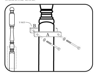
Insert bolt with washer through clamp and screw into T-nut on opposite clamp. The clamp with the T-nut should be on the outside of the post. Mount gate according to instructions.
