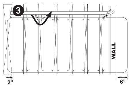
3. Hold plastic in place with ends overlapping endposts (2 inches) and/or wall (6 inches). Make marks on the plastic on either side of one of the baluster posts no less than 1/2 inch from the top edge. Use hole punch (B) to punch holes at your marks. Press hard, you may need to use both hands. Use cable ties (A) and insert through the holes from the backside of the plastic. Tighten the tie, and cut off the excess cable tie. Repeat this process on top and bottom of each baluster.
