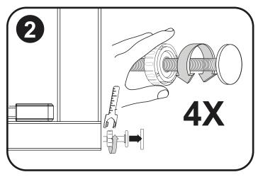
Twist to secure gate in opening. If needed, use wrench (F) to tighten.
