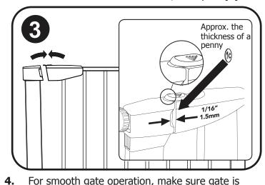
For smooth gate operation, make sure gate is level and the latch gap is only 1/16" (penny width). NOTE: Too loose or tight will cause latch to not function properly.
