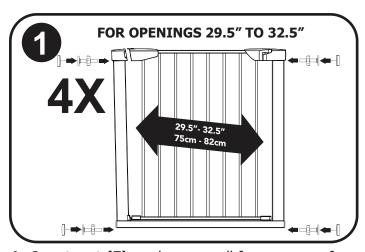
1. Insert part (E) as shown on all four corners of the gate. (Make sure flat end faces gate.)
