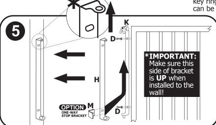
Mount latch assembly (**K**) to gate using 3/4" bolts with serrated washers (**D**). Attach wall mount for latch assembly (**H**) up into part (**K**) that is now secure on gate. Slide gate out to mark holes for (**H**) on attaching wall. (\*OPTIONAL ONE WAY BRACKET INSTALLED HERE) Then attach the wall mount of latch assembly to wall using Phillips head screws (**C**). Optional long screws (**J**) maybe be used to attach gate to stud through dry wall.
