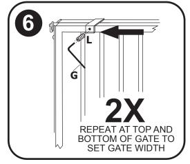
Keep gate closed and latched. Use Allen wrench (G) to insert set screws (L) in the upper and lower brackets of the gate. Tighten the set screws to set the width of the gate.
