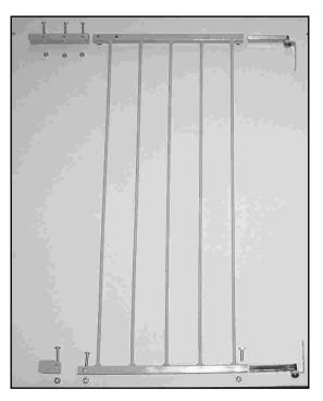
2. Connect extension to gate frame as shown using 5" connecting bracket at top with 1" phillips head bolts and lock nuts. Connect bottom using short bracket and 1/4" x 1" hex bolt and lock nuts as shown.
