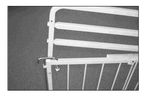
1. Rest TPX-1 on top of gate with large end toward latch. Loosely attach large end to the gate frame using #10  $\times$  1-1/2" bolt & lock nut.
