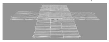
Lock the two side panels onto the back and front panels by snapping the wire hook onto the wire frame.
