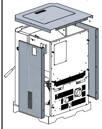
3. Once side panels have been removed, install metal brackets as shown on outside of unit.
