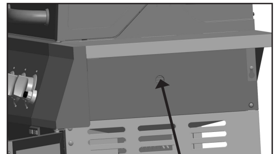
Hole for viewing the flame
