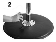
2. Use a Hex Wrench (G) to attach the Table Plate and Leg (E) to the underside of the Tabletop (D) with the provided Hex Bolts (F).
