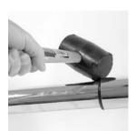
To remove the Table Top from the Support Cylinder, turn the table upside down, and strike the edge of the Support Cylinder several times where it meets the support leg of the tabletop. The Support Cylinder and Table Plate and Leg will separate with applied force.
