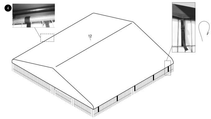
• **Note**: This Roof Cover is not meant to hold heavy snow or ice loads. Snow or ice accumulation may cause your roof cover to collapse. To avoid overload, brush snow and ice from the roof with a broom or mop.
