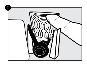
Remove the housing lid and then remove the housing by pushing in on the release tabs on both sides and lifting up.
