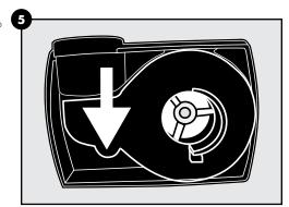
Use a fingernail to pull out the impeller (white 3-bladed propeller), which is held in place magnetically.
