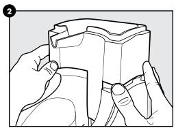
Remove the pump from the square indentation and pull the in-line plug up through the hole on the side of the bowl.
