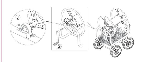
Step 7 Connect Longer Handle "H" with Short Handle Bar with Screw & Nut and Washer "J".
