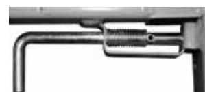
H Make sure that all four Lock Pins are secure and in LOCKED position.
