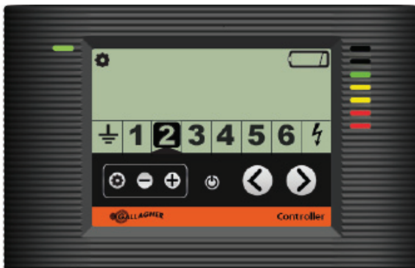
Controller showing zone 2 with a low battery
