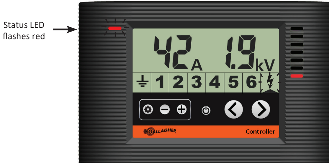
Controller showing the energizer in current alarm
