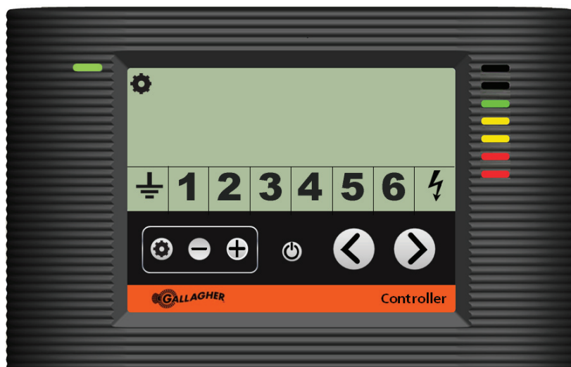
Controller showing the output voltage being adjusted
