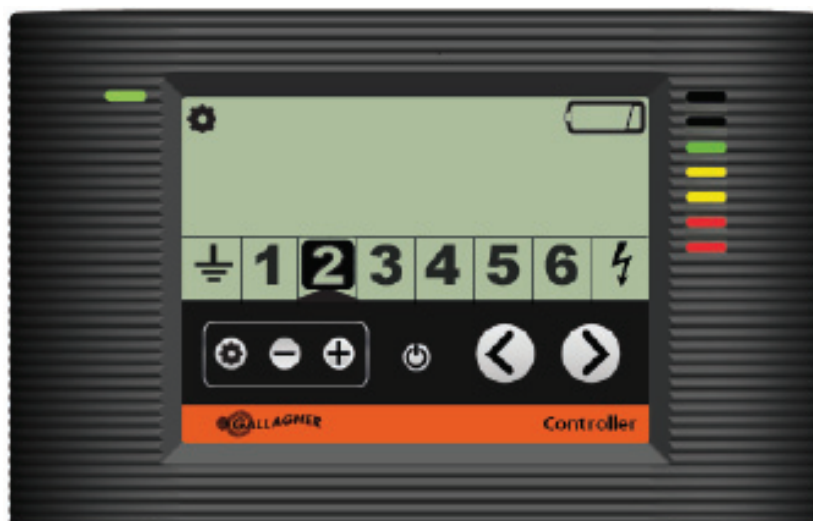
Bedieningspaneel toont zone 2 met lege batterijen
