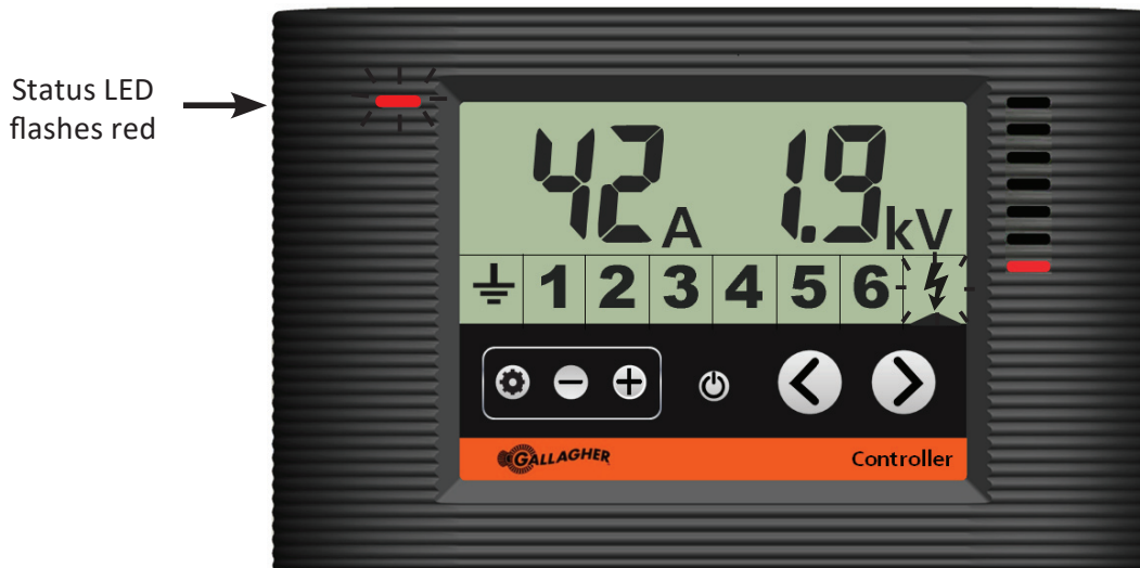
Controller showing the energizer in current alarm
