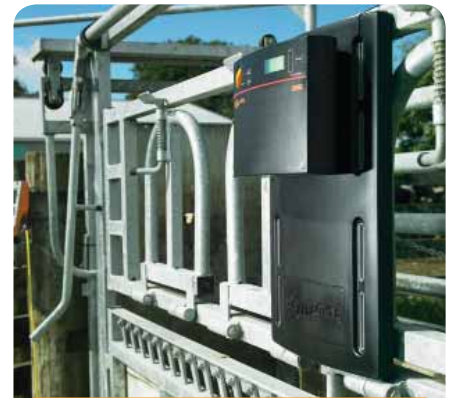
Integrated BR Series and Weigh Scale Indicator system on cattle handler.
