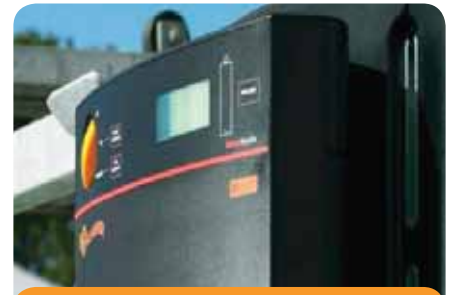
BR Series automatically provides ID number to Weigh Scale Indicator enabling accurate collection of individual sheep weights.
