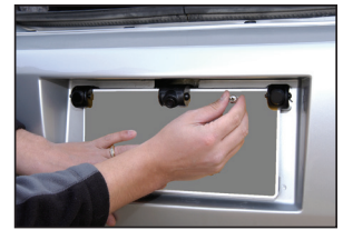
Secure license plate bracket with provided screws
