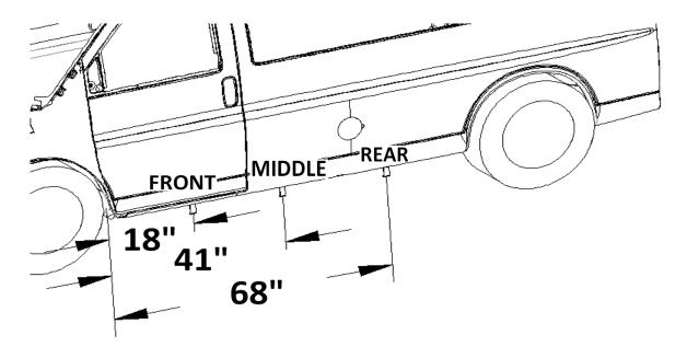
Make sure there is nothing on the bottom of the frame at these location that would obstruct the channel / angle brace from being installed in the later steps. If there is an obstruction, move the rocker panel bracket to the front/rear as needed.
