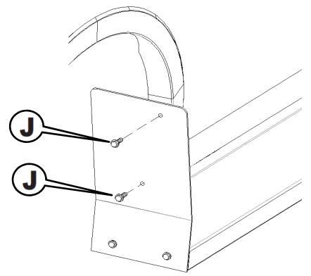
Check all hardware to make sure it has been tightened. Repeat the assembly steps for the other side of the vehicle.
