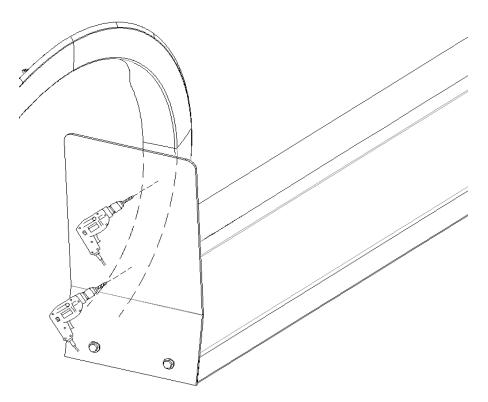
Attach the mud flap to the wheel well using two sheet metal screws [K] with a 3/8" socket. Repeat for the rear of the board.
