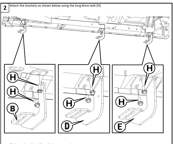
Tighten bolts with a 13mm Socket or wrench.
