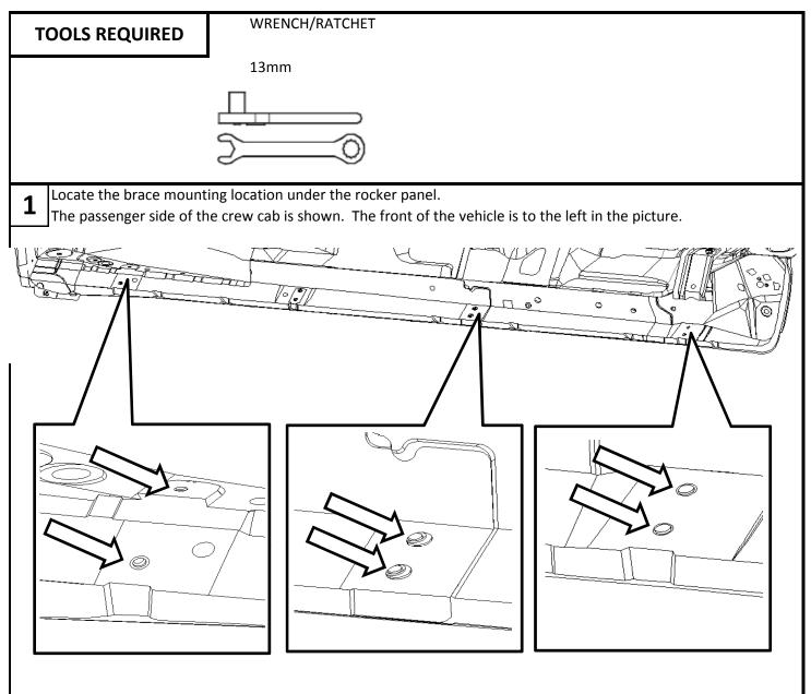
The regular cab will only have 2 mounting location. It will use the front and middle brace. For regular cab installations, the rear brace can be discarded.
