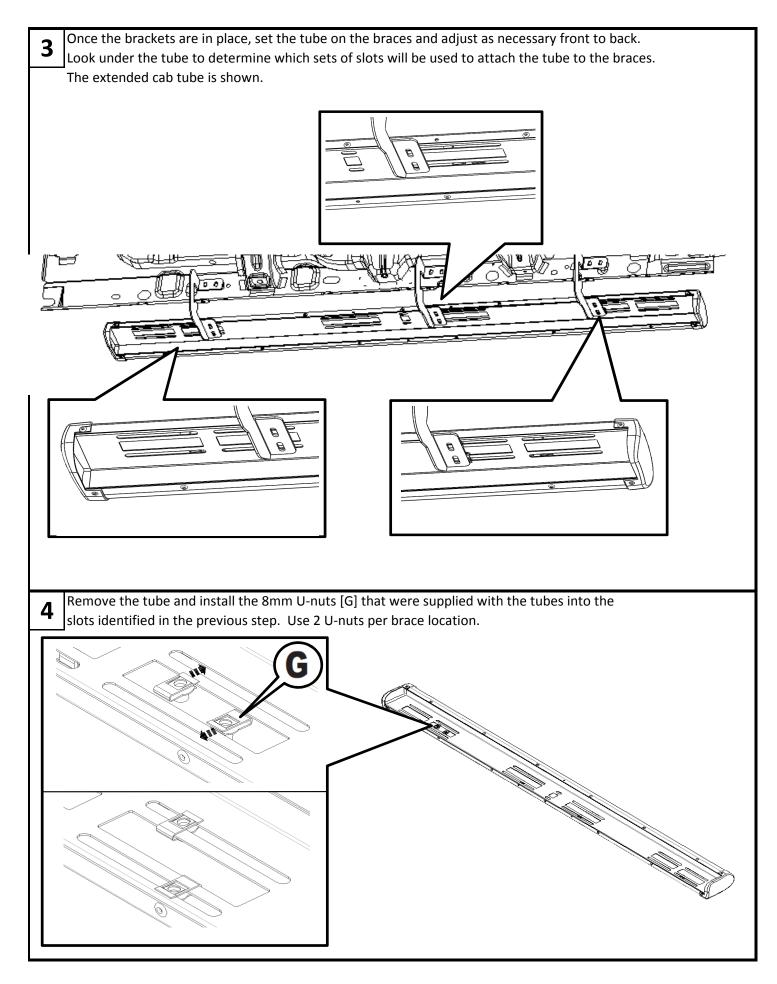
Set the tube back on the brackets and slide the U-nuts in the tube slots so that they align 5 with the mounting slots in the braces. Repeat at all mounting locations. Attach the tube to the braces using the 8mm x 20mm bolts [F] that were supplied with the tube step. Tighten bolts with a 13mm wrench or socket. Repeat at all mounting locations. ⊨∋ 0  $\bigcirc$ 0 6
