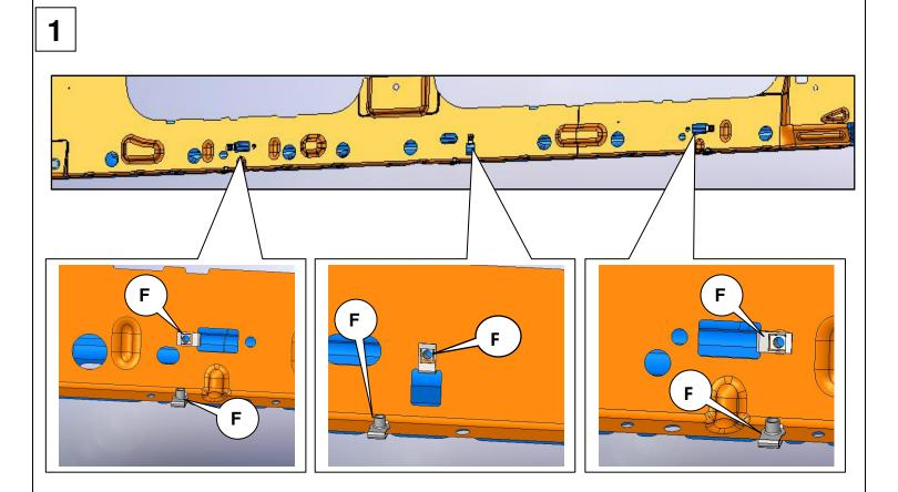
NOTE: FOR STANDARD CAB APPLICATIONS, MIDDLE BRACKET LOCATION IS NOT AVAILABLE. PROCEED AS DIRECTED USING FRONT AND REAR MOUNTING LOCATIONS. EXTRA BRACKETS AND HARDWARE MAY BE DISCARDED.
