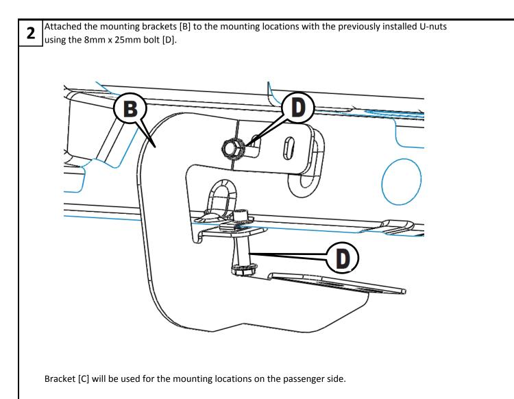
Tighten bolts with a 13mm Socket and wrench.
