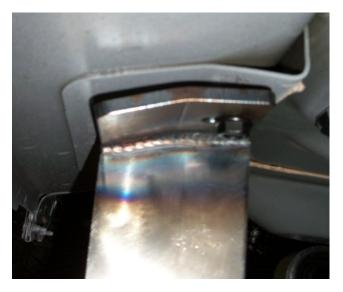
While pulling down on the front brace, tighten the long bolt with a 13mm socket. Then tighten the short bolt with a 13mm socket.
