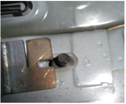
Align the other slot in the brace with the small threaded plate in the square hole opening. Attach with the short 8mm bolt [I] and washer [C], but do not tighten at this time.
