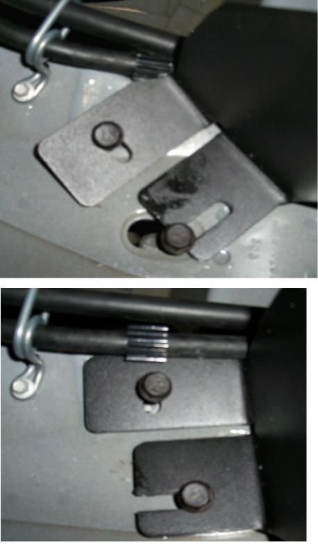
While pulling down on the brace, tighten the bolts with a 13mm socket.
