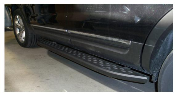
Attach the board to the braces using the flange nut [K]. Tighten all bolts with a 13mm socket.
