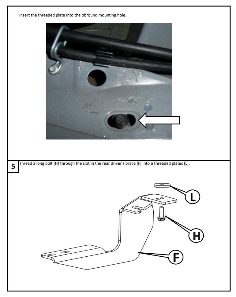
Insert the threaded plate into the round mounting hole. Then rotate the brace so the open end slot in the brace captures the previously installed threaded plate.
