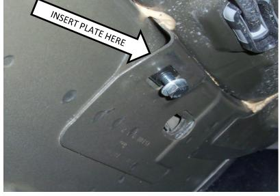
NOTE: THE BOLT WILL NOT ACTUALLY BE IN THE PLATE WHEN IT IS INSTALLED. IT IS SHOWN HERE TO HELP MAKE CLEAR WHERE THE THREADED PLATE WILL GO.
