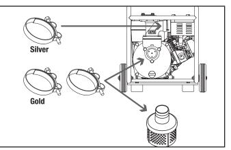
**Gold (2) : 54-57 mm ID clamp** – For green suction hose connection to pump inlet port (center of pump and intake screen).
