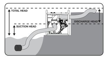
Pump output will be affected by the type, length, and size of the suction and discharge hoses. The pumping height, also known as the total head, is the distance from the water level to the point of discharge. As this distance increases, pump output decreases.
