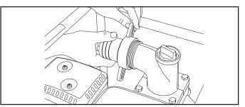
Slide the blue discharge hose over the discharge fitting (top of pump) and secure with the hose clamp (52-55 mm ID) with wrench.
