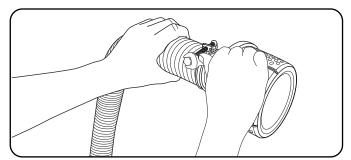
Remove the top cap from the pump chamber and completely fill the chamber with clean water. Tighten the cap. DO NOT over tighten.
