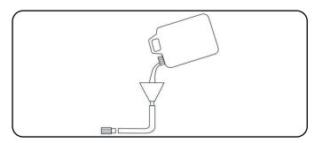
5. Pour the antifreeze into the funnel, then pull on the engine recoil starter to create suction in the pump housing. Pull the recoil several times until antifreeze comes out of the pump outlet. DO NOT START THE ENGINE WHEN DOING THIS. Only pull the recoil cord if the fuel valve and engine switch are in the OFF position.
