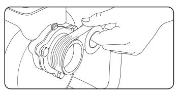
5. Attach the quick coupler to the male coupler and lock in place with the cam lock.
