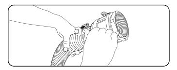
4. Wrap the 2 in. (5.1 cm) NPT inlet clockwise with the Teflon<sup>®</sup> tape provided. Carefully thread the male connector to the intake port.
