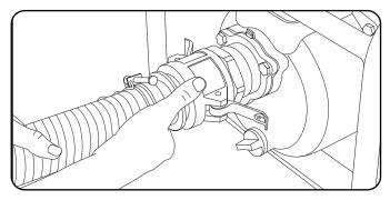
6. Attach the strainer to the intake hose and secure with the hose clamp.
