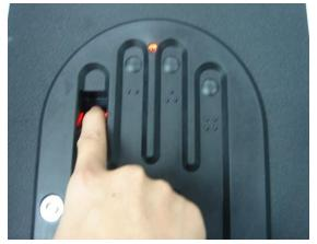
Now the first fingerprint is enrolled. (Up to 15 users can be enrolled)
