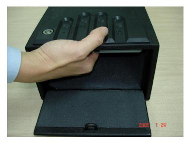
• Press and hold the Learn Button a third time for two seconds. Release the Learn button. The light will blink green five times. And you will hear five beeps, confirming that the new code has been accepted. If the red light blinks three times with three soft beeps at this point, and error has occurred. Just start over by depressing the Learn Button for two seconds.
