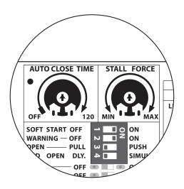
Do not use the Dual Sense Stall Force adjustment to compensate for a gate that is sticking or binding. Excessive Stall Force may cause damage to the gate operator or gate system or Injury or Death.
