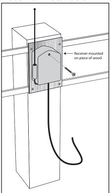
Check the range of the receiver *before permanently mounting* it. You may have to try different locations before permanently mounting the receiver. The receiver range can vary from 50 to 100 feet depending upon weather, topography, and external interference.
