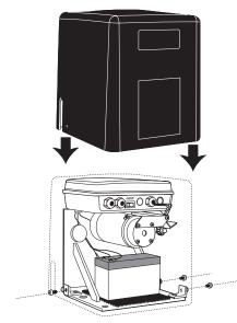
Mount the operator housing after all installation procedures are complete. Slide operator housing over legs, align holes, and use screws provided to attach housing to operator.
