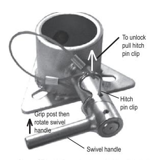
Photo of Triangle Base showing swivel handle locked with hitch pin clip installed. To unlock, pull hitch pin clip upward until removed. Firmly grip jack post before rotating swivel handle 180 degrees. The hitch pin clip MUST be installed at all times except when using the rapid deployment feature of the RDJ-2K as explained above.
