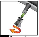
Remove valve core with included tool.
