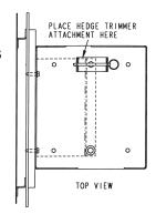
**1.** Assemble the gusset bracket and hedge trimmer bracket (if used) to the multi-rack weldment with two 3/8-16 x 1-1/4 screws, flat washers and nuts supplied. If the hedge trimmer bracket is used, omit the washer under the head of the screw that holds it.
