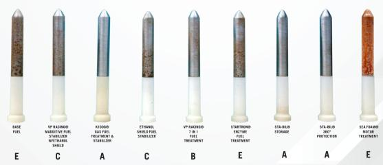
\* CORROSION CONTROL TEST IS AN ACCELERATED CORROSION TEST BASED ON A MODIFICATION OF THE NACE TM 0172 TEST PROTOCOL, REPLACING DISTILLED WATER WITH SYNTHETIC SEA WATER PER ASTM D665 PART B. SYNTHETIC SEA WATER IS MORE LIKELY TO CAUSE CORROSION THAN DISTILLED WATER. UNITECTED CARBON STEEL RODS DEPICTED PLACED IN A BASE FUEL BIELD OF ELIO GADIO, SEADON, SYNTHETIC SEA WATER FOR 4 HOURS. GRADES, "C" AND BELOW FAIL THE STANDARD. TESTING AND GRADING PERFORMED BY INDEPENDENT STANDARD STANDAR
